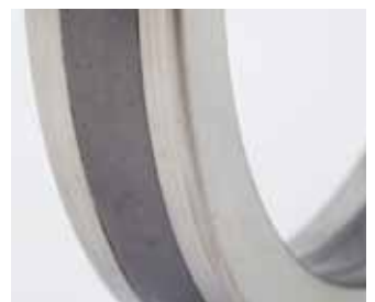
Composite ring consisting of a central ring of expanded graphite with compressed braided rings at the ends. The set provides a perfect sealing up to 1000 bar.
